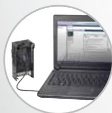
**Simplified Programming** – MainsFree™ programming allows configuration files to be uploaded and downloaded to the PowerFlex 525 and PowerFlex 523 drive control module via a USB connection.
